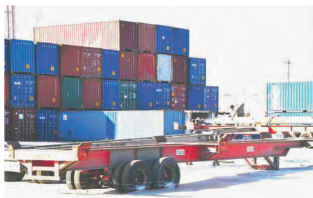
Fig. 6. Another documentation that the sand and water spouts in the port started before the strong ground shaking (please note the two parallel horizontal white signs on the tires which are due to bounding of the lorry platform on the ground during the strong phase of the ground motion. The ejected material was already there).
