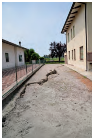
Fig. 13. Lateral spreading in San Carlo, with ejected liquefied grey fine sand material in residential area. Ground cracks with opening of about 20cm, vertical offset of 10-20cm and local extensional strains is evident.
